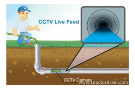
1. Detailed Inspection and Diagnosis: Using advanced video inspection technology, we can see exactly what's going on inside your pipes. This allows us to pinpoint the cause of the problem, whether it's tree roots, grease buildup, rust, or a broken pipe. For new homeowners, this service is especially valuable, as it provides a clear assessment of the plumbing's condition.
